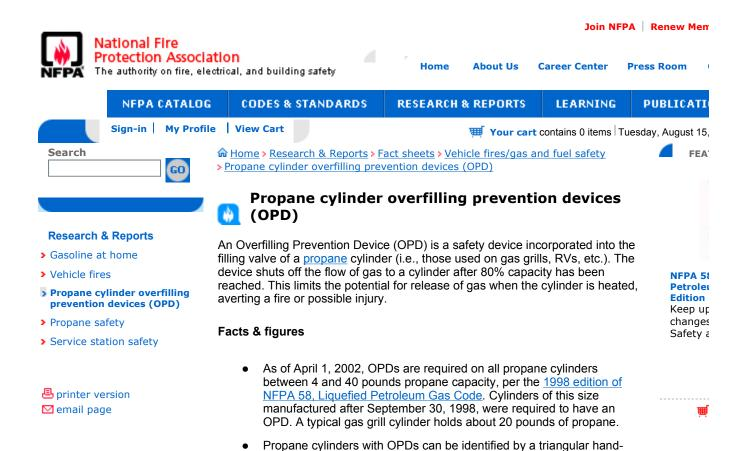
After April 1, 2002, propane cylinders not equipped with an OPD must be retrofitted with the device before refilling can occur or properly disposed of and replaced with an OPD-equipped cylinder.
