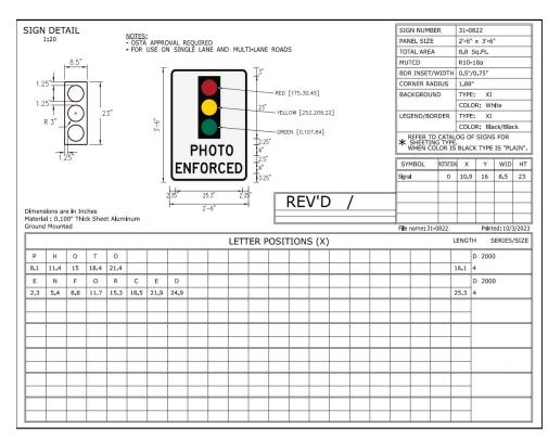
Sign detail options for "Photo Enforced" to be installed at a traffic control signal
